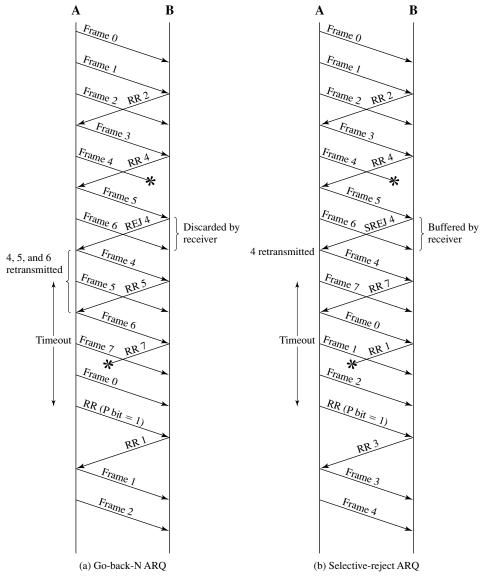
Figure 7.6 Sliding-Window ARQ Protocols
