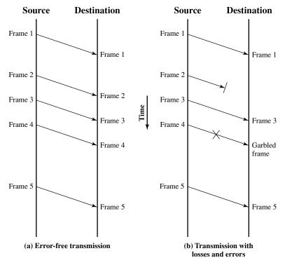
Figure 7.1 Model of Frame Transmission
