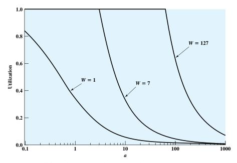
Figure 7.12 Sliding-Window Utilization as a Function of *a*
