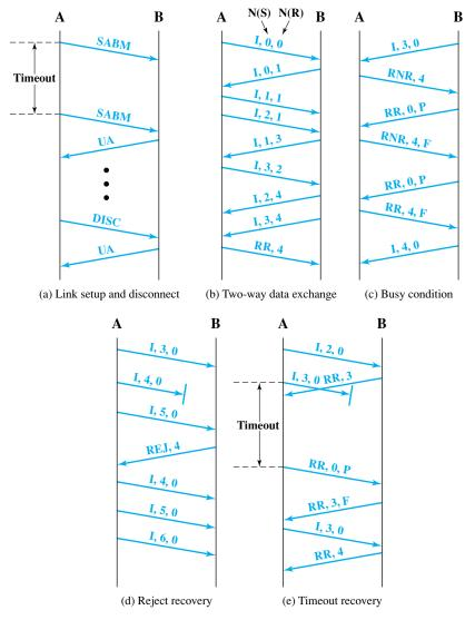
Figure 7.9 Examples of HDLC Operation
