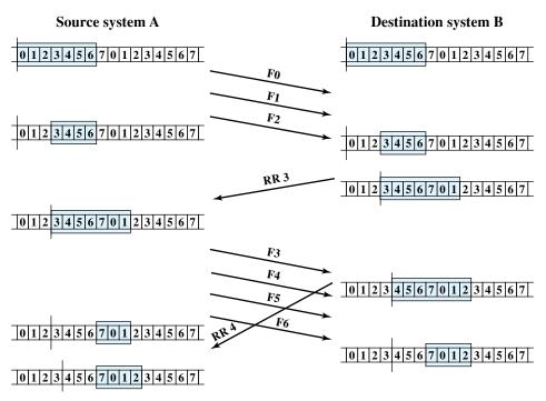
Figure 7.4 Example of a Sliding-Window Protocol
