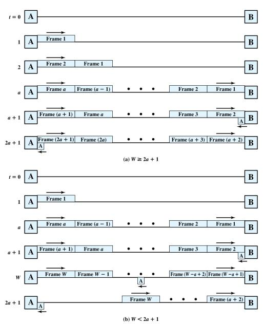
Figure 7.11 Timing of Sliding-Window Protocol
